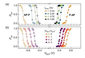
FIG. 4. Probability of AP-P (open symbols) and P-AP (full symbols) switching measured post-pulse as a function of  $V_{\rm SOT}$ . (a) Switching at  $V_{\rm MTJ} = 0$  for different pulse widths and (b) switching at different  $V_{\rm MTJ}$  for  $t_{\rm pulse} = 0.33$  ns.
