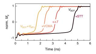
FIG. 7. Simulated switching traces for AP-P reversal induced by  $j_{\rm SOT} = 81 \,{\rm MA/cm^2}$  without (black line) and with (yellow line) MTJ bias given by  $V_{\rm MTJ}/V_{\rm SOT} = -0.9$ , and taking into account only one bias-induced effect at time (orange-red lines).
