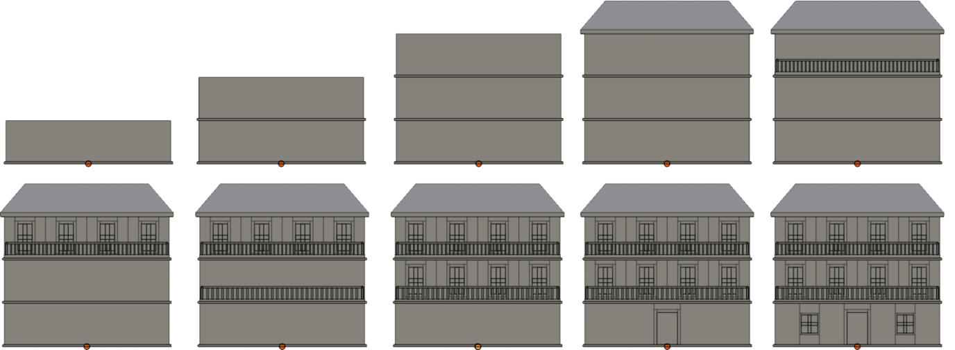
Fig. 6: Mesh generation for a 3d building model. We start from the silhouette of each floor, and then gradually add its elements.
