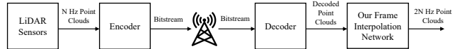
Fig. 3. The illustration of the application into reducing the amount of the point cloud transmission.
