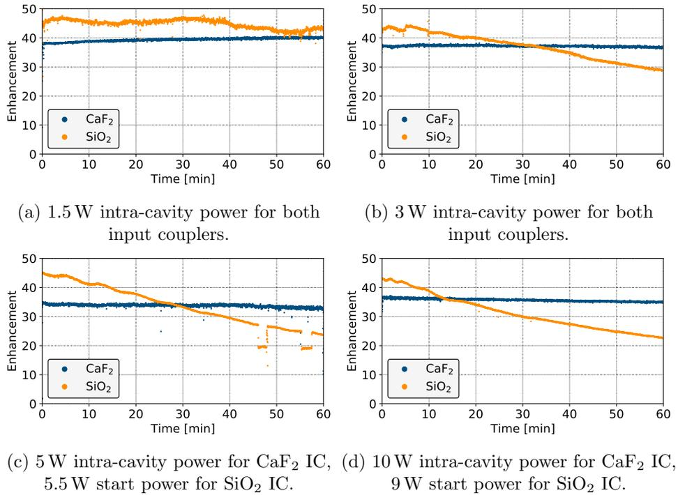
Figure 3: Enhancement versus time of CaF<sub>2</sub> IC versus SiO<sub>2</sub> IC for different intracavity powers at  $10^{-8}$  mbar.
