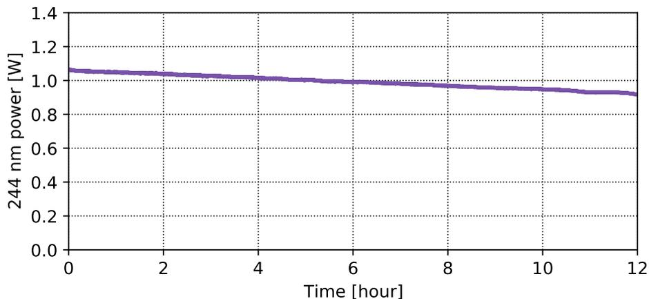
Figure 2: Performance of the 244 nm laser system over long time scales. The laser can output 1 W of 244 nm power over several hour time scales without degradation of the CLBO crystal. We attribute the slow degradation observed to damage of the output coupler.
