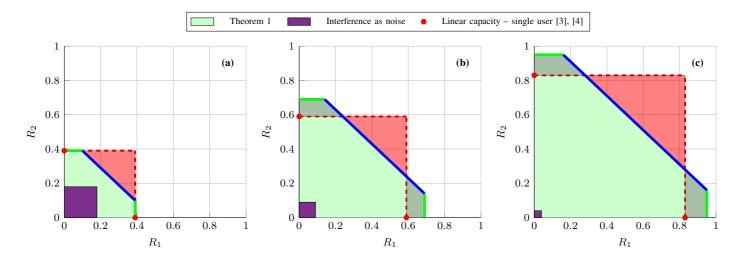
Fig. 3: Outer bound rate regions for a transmitted power per user of (a) -2.9 dBm, (b) 0 dBm, and (c) 2 dBm.
