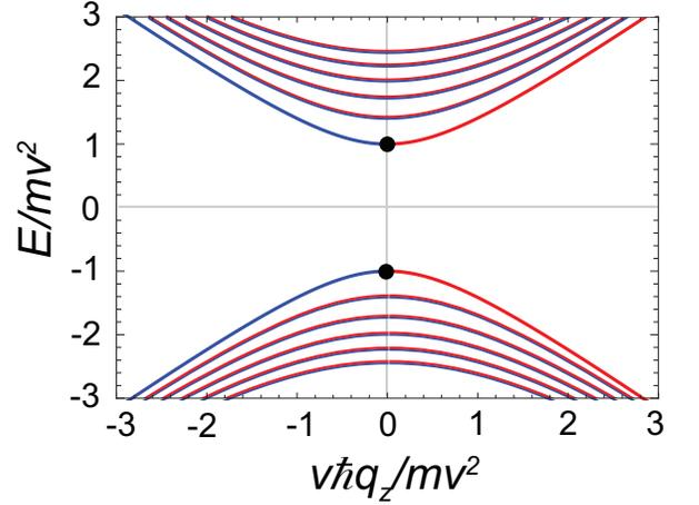
Figure 1. The energy dispersion spectrum of the Landau levels with helicity distribution (blue line for right handed and red for left handed helicity). The two black dots indicate the discontinuity of helicity in the Landau levels of  $n = 0$ .
