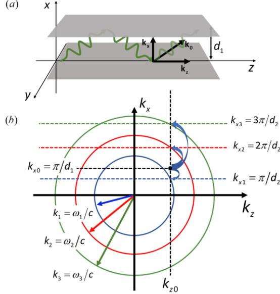
Fig. 2. (a) Representation of the propagation quantities of the TE/TM modes within a parallel-plate waveguide of dimension  $d$ . (b) Dispersion diagram of the excited modes supported by the waveguide after a temporal discontinuity induced by a sudden change of the waveguide dimensions from  $d = d_1$  to  $d = d_2$ .
