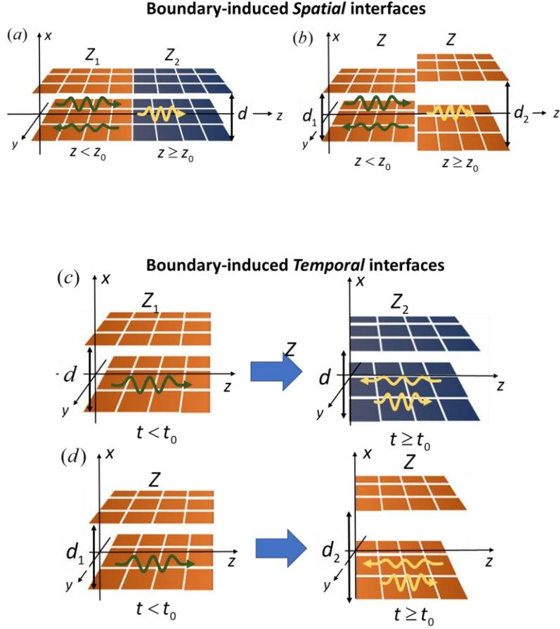
Fig. 1. Graphical illustration of the wave propagation discontinuities induced by the boundaries in a guiding structure: (a) spatial and (c) temporal interfaces induced by a change of the bounding surface impedance; (b) spatial and (d) temporal interfaces induced by a change in the separation between waveguide plates.
