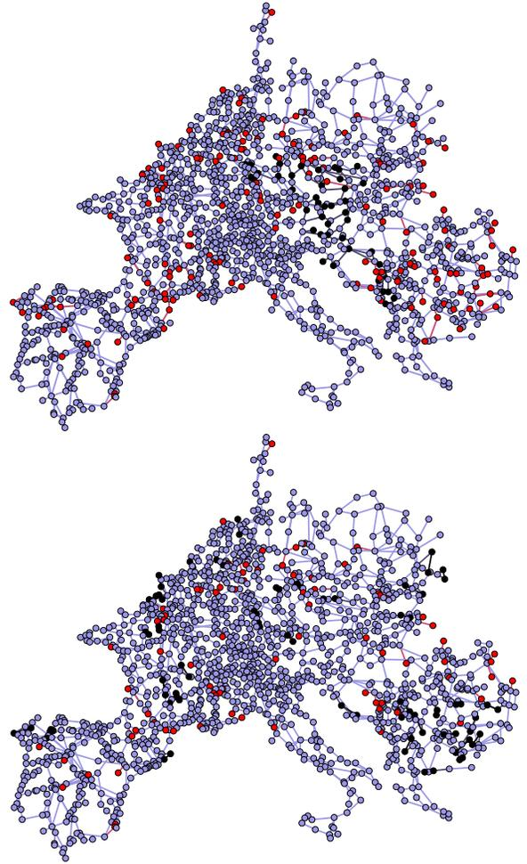
**Fig. 2:** (top) The European power grid with 151 unmatched bus-nodes (shown in red) whose states need to be measured via PMUs. An example contraction of 46 nodes is also shown in black. (bottom) By adding 40 edges (shown in black) to increase the GCC of power network, the number of unmatched bus-nodes (and minimum required PMUs) is reduced to 80.
