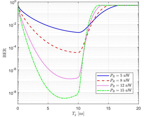
Fig. 5. BER versus the gate-ON interval  $T_g$  for a small time-gated SPAD array with  $N = 64$  under various received signal power  $P_R$  when  $P_b = 7$  nW and data rate  $R = 50$  Mbps.
