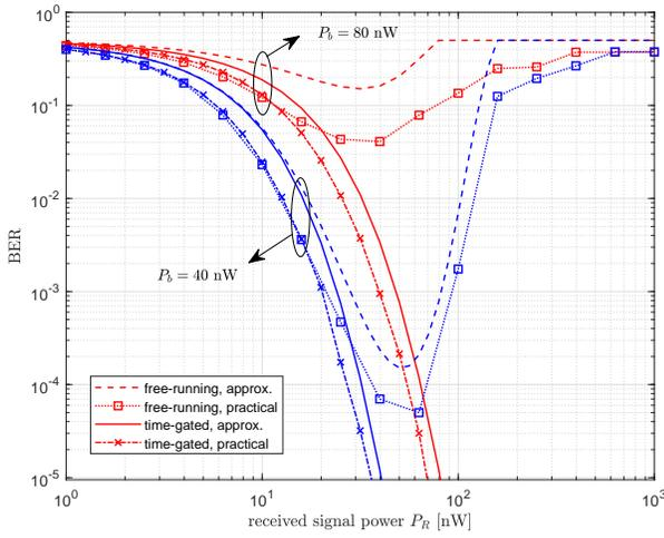
Fig. 10. BER versus the received signal power  $P_R$  for a large SPAD array with  $N = 1024$  and data rate  $R = 200$  Mbps under various background light power  $P_b$  in the presence and absence of the gating operation.
