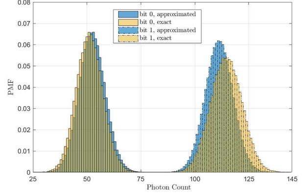
Fig. 4. The exact and approximated conditional PMFs of the detected photon count when bit ‘0’ and bit ‘1’ are transmitted where  $\lambda_0 = 2 \times 10^7$  Hz,  $\lambda_1 = 7 \times 10^7$  Hz,  $T_d = 10$  ns,  $T_s = 50$  ns and the number of SPAD  $N = 64$ .
