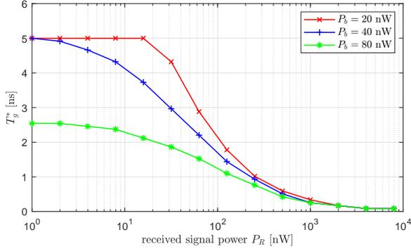
Fig. 9. The optimal  $T_g$  versus the received signal power  $P_R$  for a large SPAD array with  $N = 1024$  and data rate  $R = 200$  Mbps under various background light power  $P_b$ .
