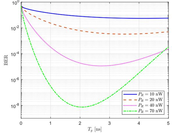
Fig. 8. BER versus  $T_g$  for a large time-gated SPAD array with  $N = 1024$  under various received signal power  $P_R$  when  $P_b = 40$  nW and data rate  $R = 200$  Mbps.
