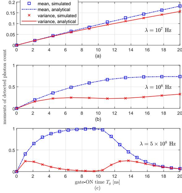
Fig. 3. The mean and variance of the detected photon count versus the gate-ON time  $T_g$  for time-gated SPAD under various incident photon rate  $\lambda$  with dead time  $T_d = 10$  ns and symbol time  $T_s = 20$  ns.
