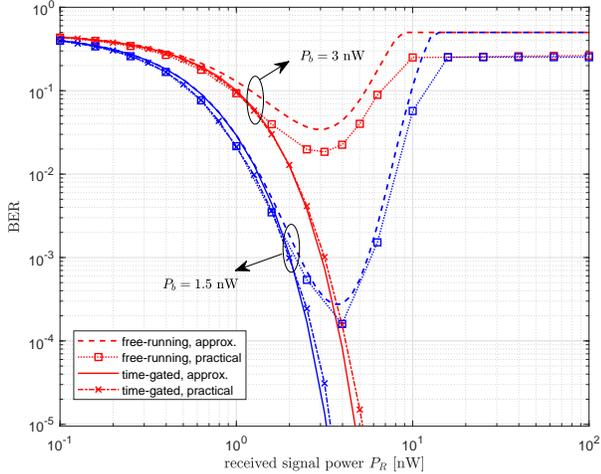
Fig. 7. BER versus the received signal power  $P_R$  for a small SPAD array with  $N = 64$  and data rate  $R = 50$  Mbps under various background light power  $P_b$  in the presence and absence of the gating operation.
