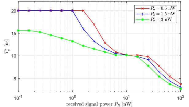
Fig. 6. The optimal  $T_g$  versus the received signal power  $P_R$  for a small SPAD array with  $N = 64$  and data rate  $R = 50$  Mbps under various background light power  $P_b$ .
