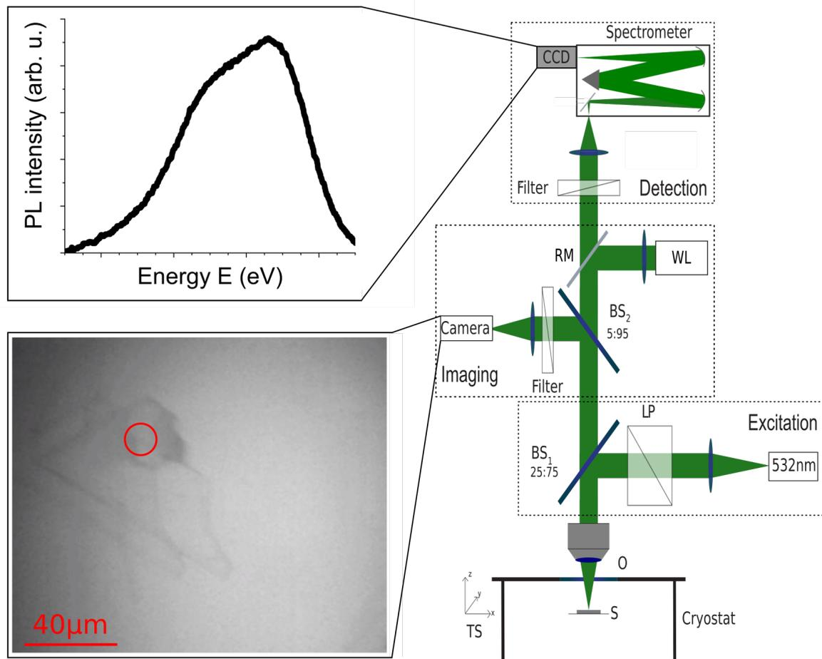
**Figure S3.** Simplified schematic of the  $\mu$ -PL setup with an exemplary PL spectrum and microscope image of the exfoliated and hBN encapsulated WS<sub>2</sub> monolayer. The red circle highlights the monolayer position.
