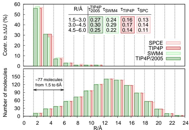
Figure 3. Top: Contribution of the solvent atoms with their center of mass at the respective distance  $R$  to the closest oxyquinolinium atom to the overall magnitude  $\Delta\Delta U$ . The inset lists an estimate of the mean relaxation times  $\langle\tau\rangle$  of the water molecules in the three bins that contribute most to the shift. Bottom: Number of solvent molecules at the respective distances.
