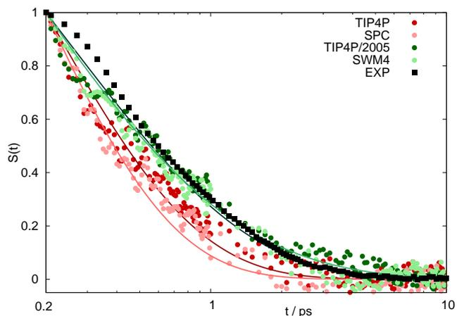
Figure 4. Comparison of experimental (EXP) data, extracted from Ref. [4], with the Stokes shift of 1MQ in SPC and SWM4 water using the CHelpG  $\omega$ B97xD partial charge distribution from calculations in implicit solvent. Solid lines represent the respective fitted Kohlrausch/Gaussian functions (see Eq. (9)).
