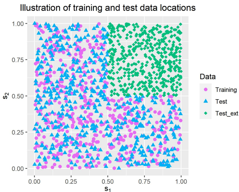
Figure 1: Example of locations for training and test data for the spatial data. “Test” and “Test_ext” refers to locations of the “interpolation and “extrapolation” test data sets, respectively.
