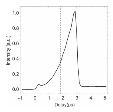
**Figure S1.** Intensity envelope of the narrowband field used in the FSRS probe, as obtained from two-photon absorption measurements in the  $50 \mu m$  thick LiNbO<sub>3</sub> sample. The dashed line indicates the fixed position of the white light continuum pulse during the FSRS measurements.
