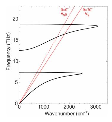
**Figure S2.** Black curve: Dispersion relation for the c-axis modes in LiNbO<sub>3</sub> plot using parameters obtained from Ref. 36. The slope of the dashed red curve indicates the group velocity of a pulse with carrier wavelength of 400 nm, and the solid red curve indicates the effective group velocity of such a pulse propagating at an angle of 30° relative to the polariton.
