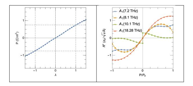
**Figure S3.** Left Panel: Total polarization as a function of structural distortion going from the  $-P_0$  ferroelectric state to the inverted  $+P_0$  state crossing the centrosymmetric state in the middle. Right panel: Raman tensor of the four polar  $A_1$  modes in LiNbO<sub>3</sub>
