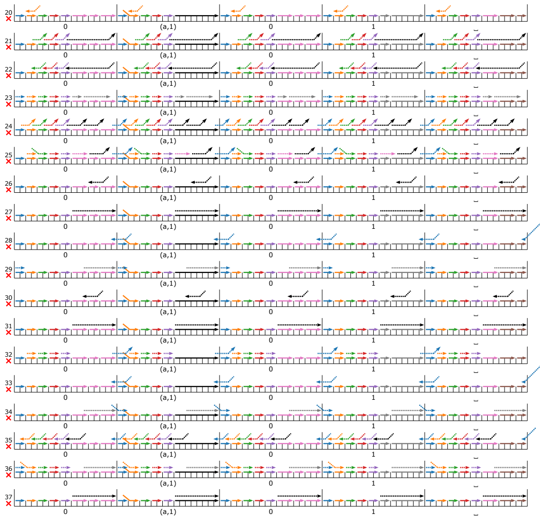
Figure 16 An overview of instructions 20 to 37 of the construction, which represent the (a, 1) \rightarrow (a, 1, R) transition of the Turing machine shown in Figure 3. Because the register in this example is not in the (a, 1) configuration, the instructions in this section do not affect the register, as no toehold is present.
