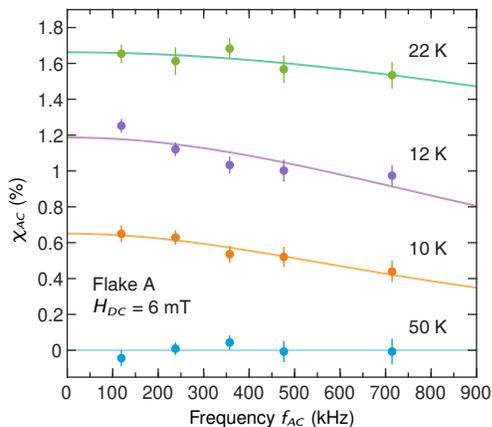
FIG. 5. Frequency-dependent susceptibility of domain walls in ultrathin CrBr<sub>3</sub>.  $\chi_{AC}$  for Flake A at 50 K (blue), 22 K (green), 12 K (purple), and 10 K (orange) during FC. The solid lines are fits using a damped, driven domain wall oscillation model. The number of  $\pi$ -pulses increases for larger  $f_{AC}$  (e.g., XY8-N6 is used for 714 kHz).
