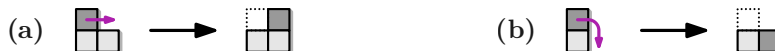
■ Figure 1 Moves admitted by the sliding cube model: (a) slide, (b) convex transition.
