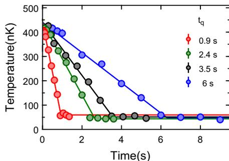
FIG. S1. Evolution of the sample temperature in the quenching for various quench times  $t_q$ . The solid lines are bilinear fits to the data for each  $t_q$ , where the later line segments are kept horizontal. Each data point was obtained from ten measurements of same experiment, and its error bar represents the standard error of their mean.
