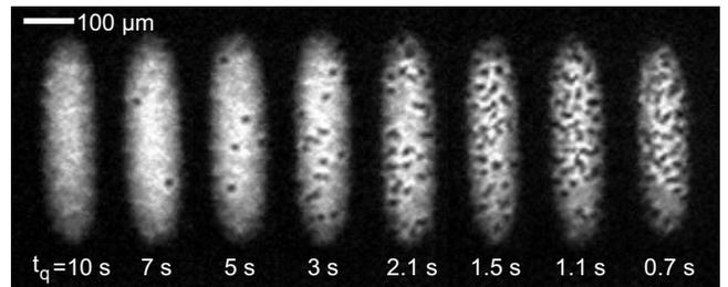
FIG. 1. Spontaneous defect formation in an atomic Bose gas quenched into a superfluid phase. A sample is cooled by linearly decreasing the trap depth for variable quench time  $t_q$ . Images of the gas for various  $t_q$ , obtained after a time-of-flight, where quantum vortices generated during the phase transition are detected by their expanded, density-depleted cores.
