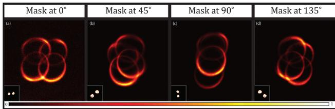
FIG. 5. Type II SPDC emission with a 2-aperture mask. The rotation of the mask demonstrates the full angular control of the emission.
