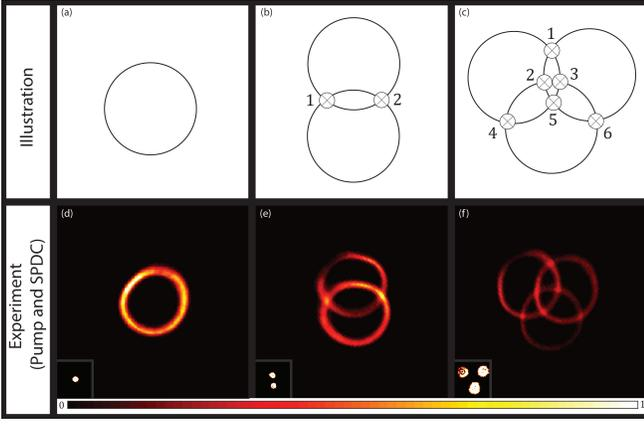
FIG. 3. (a)-(c) Illustrations of repeated Type I SPDC cones generated by a single, double, and triple "sub-Gaussian" pump, with the desired overlap labeled. (d)-(f) The corresponding experimental results obtained using GMs designed with 1, 2, and 3-apertures. For each case the pump beam was imaged and inset with the SPDC emissions. While there are no intersection in a), the entire ring is entangled due to its origin from both type I BBOs.
