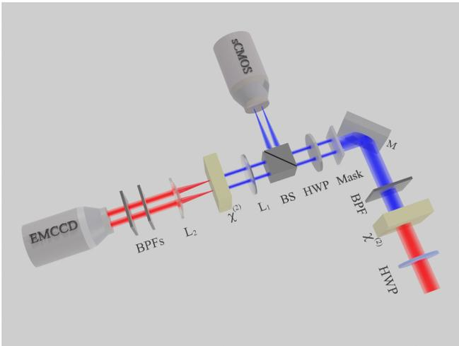
FIG. 2. Schematic of setup including Half-Wave Plates (HWP), BBOs ( $\chi^{(2)}$ ), Band Pass Filters (BPF), Beam Splitter (BS), Mirrors (M), lenses (L), and our beam masks. The sCMOS and EMCCD image the pump and down converted light respectively.
