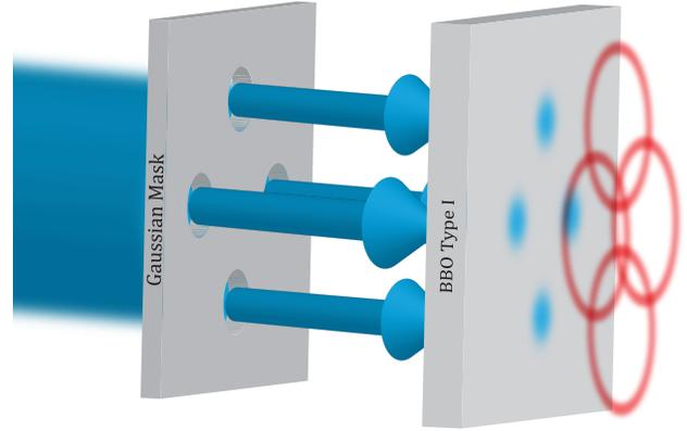
FIG. 1. A 4-aperture Gaussian mask (GM) is illustrated. Each ‘sub-Gaussian’ input generates its own SPDC emission cone. The GM design controls the number and the manner of overlap of the down-converted cones
