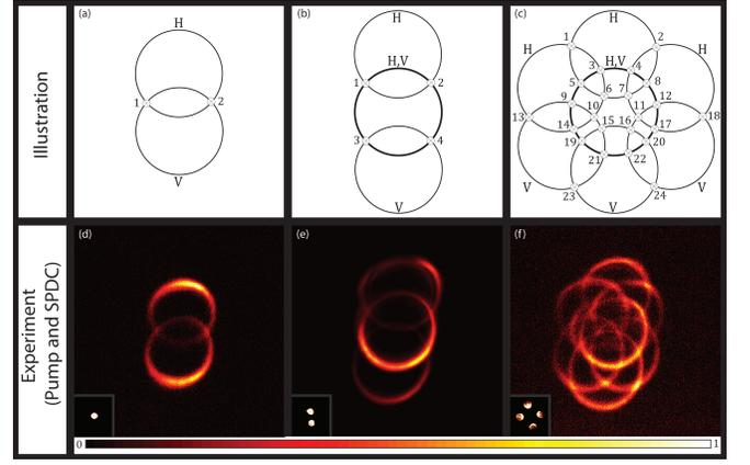
FIG. 4. (a)-(c) Illustrations of Type II SPDC cones generated by a single, double, and quadruple "sub-Gaussian" pump, with the desired overlap labeled. (d)-(f) The corresponding experimental results obtained using GMs designed with 1, 2, and 4-apertures. For each case the pump beam was imaged and inset with the SPDC emissions. In (f) the center ring is composed of overlapping rings from the emissions from both the top and bottom apertures.
