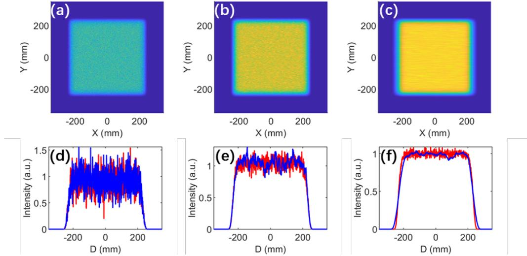
Fig. 3. The near field beam profiles of the input and output pulses of the AFGC. Input beam profile (a), and its intensity curves (d) at spatial positions  $Y=0$  (blue curve) and  $X=0$  (red curve). Output beam profile (b) and its intensity curves (e) at spatial positions  $Y=0$  (blue curve) and  $X=0$  (red curve) at  $d\theta=10$  mm. Output beam profile (c) and its intensity curves (f) at spatial positions  $Y=0$  (blue curve) and  $X=0$  (red curve) at  $d\theta=60$  mm.
