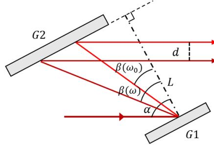
Fig.2. Spatial dispersion introduction by a pair of gratings. G1-2, diffraction gratings.  $\alpha$ , incident angle.  $\beta(\omega)$  and  $\beta(\omega_0)$ , diffraction angles of the frequencies  $\omega$  and  $\omega_0$ , respectively.  $L$ , perpendicular length of G1 and G2.  $d$ , amount of spatial dispersion.
