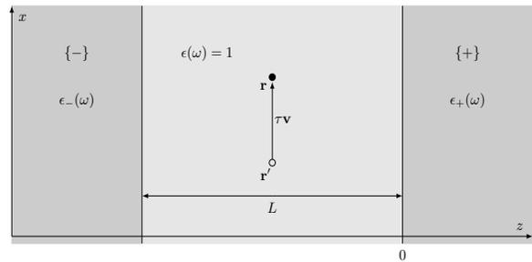
FIG. 1. The two-plate set-up, with the atom in the centre of the cavity.
