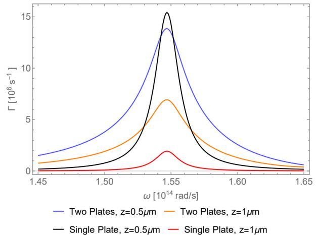
FIG. 4. The medium-induced transition rates for a static atom a distance  $z$  from one or two dielectric plates as labeled, shown for two possible atom-plate separations.
