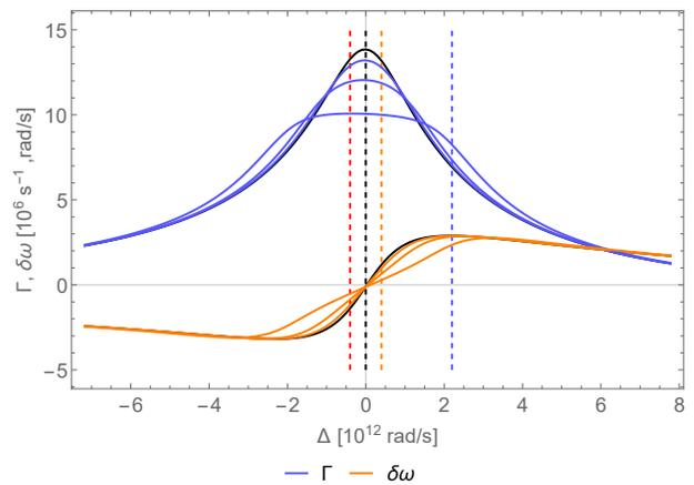
FIG. 2. Plot of the resonant contributions to the medium-induced atomic transition rate  $\Gamma$  and frequency shift  $\delta\omega$  as a function of the detuning  $\Delta$  for a static atom in the centre of two plates of separation  $1\mu\text{m}$ . The black line represents the static case, with the successively broadened  $\Gamma$  and  $\delta\omega$  profiles for  $v = 10^{-3.5}c$ ,  $10^{-3.2}c$  and  $10^{-2.9}c$  respectively.
