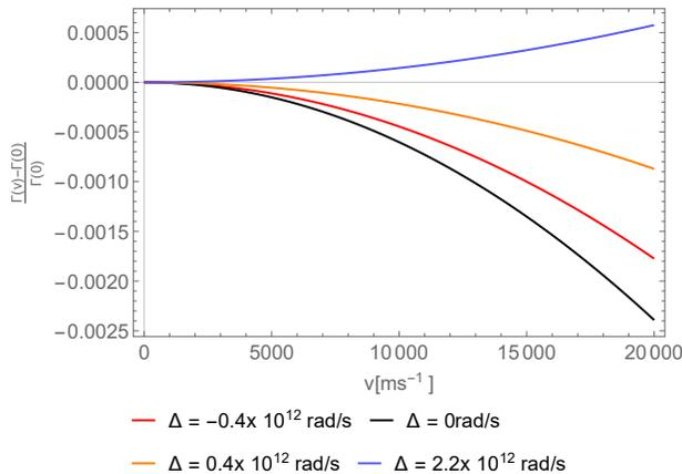
FIG. 3. The velocity dependent transition rates proportional to the static rates evaluated for 4 different detunings  $\Delta$  from the resonance.
