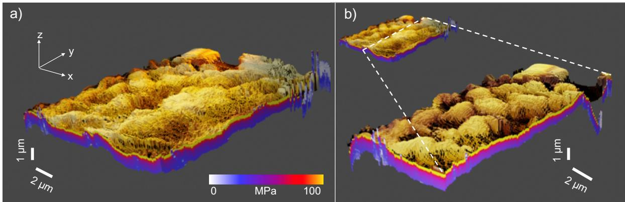
Figure 4: a) 3D representation of the surface profile of a PF. The colour in the z-direction encodes the local stiffness beneath the surface. b) A cross-sectional profile of  $E_{lok}(z)$  in the xz- and yz-directions as indicated.
