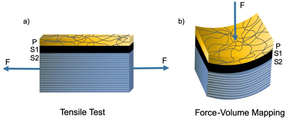
Figure 9: Fibril orientation in the applied load direction in a) the tensile test and b) force-volume mapping.
