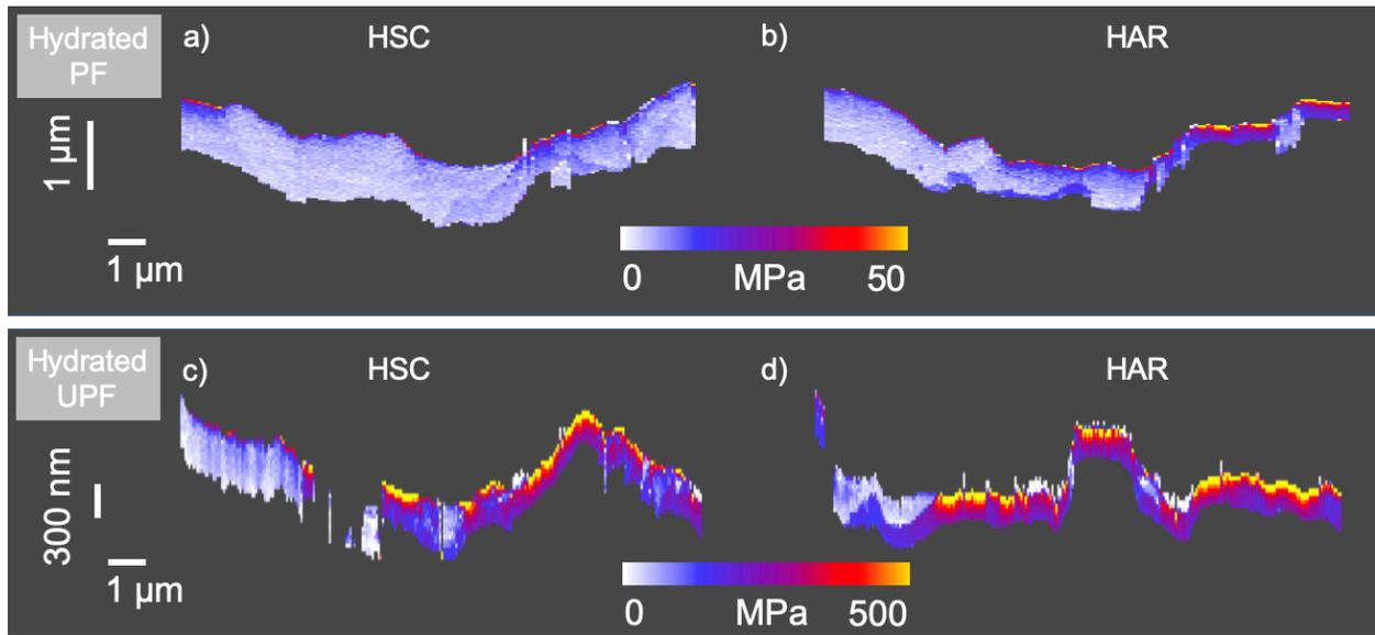
Figure 10: Cross section of  $E_{lok}(z)$  in the  $xz$ -direction of a hydrated PF mapped with a) an HSC cantilever and b) an HAR cantilever. Cross section of  $E_{lok}(z)$  in the  $xz$ -direction of a hydrated UPF mapped with c) an HSC cantilever and d) an HAR cantilever.
