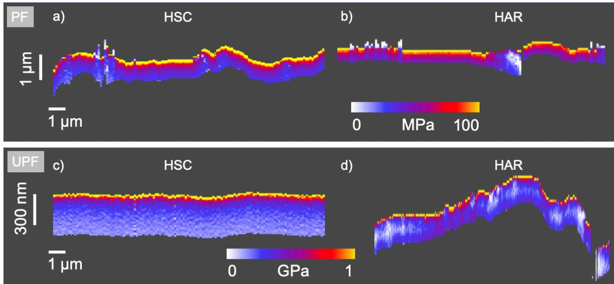
Figure 5: Depth profile of  $E_{lok}(z)$  in the  $xz$ -direction of a PF mapped with an HSC cantilever in a) and an HAR cantilever in b) and of UPF mapped with an HSC cantilever in c) and an HAR cantilever in d).
