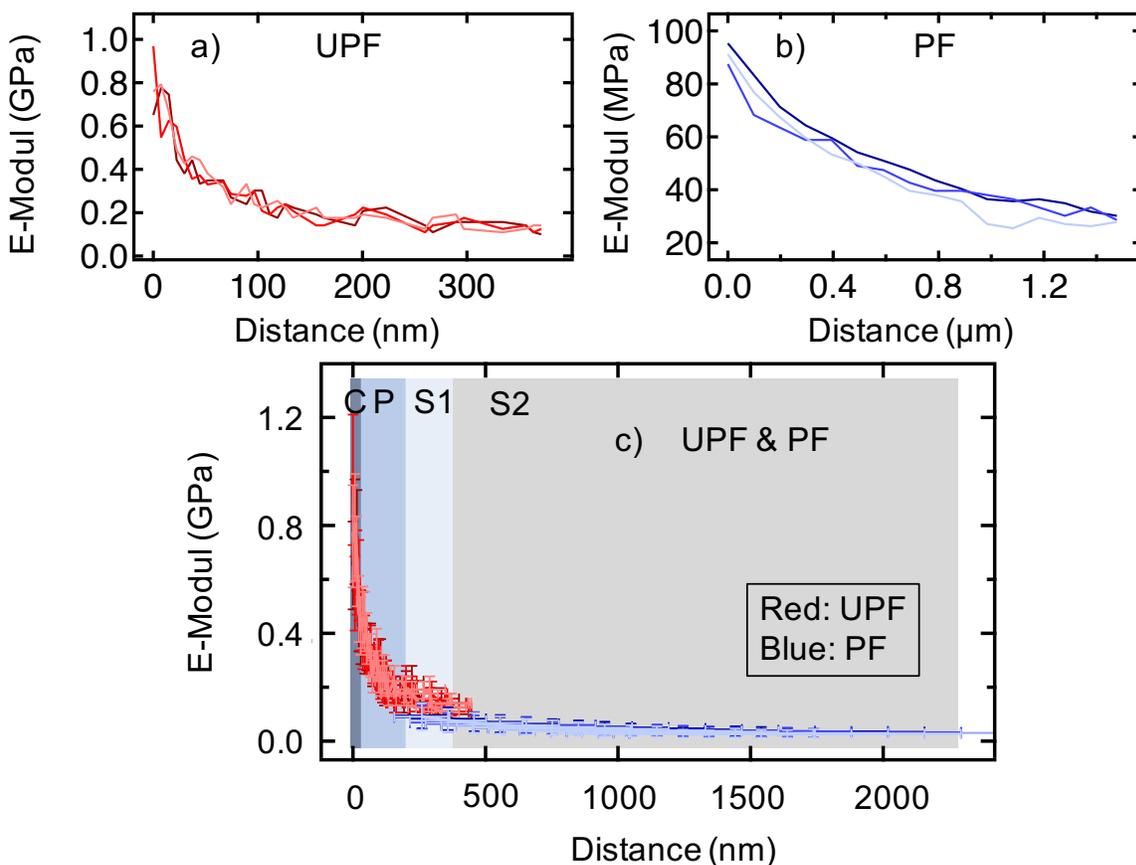
Figure 6: Depth profiles of this  $E_{lok}(z)$  of a) a UPF, b) a PF and c) a combined graph of UPF and PF. In c), the UPF profiles are plotted in red, and the PF profiles are plotted in blue. The suggested corresponding wall layers are indicated with different colours. The C layer is highlighted in dark blue, the P wall in blue, the S1 layer in light blue and the S2 layer in grey. The error bars are  $\pm 30\%$  of the values.
