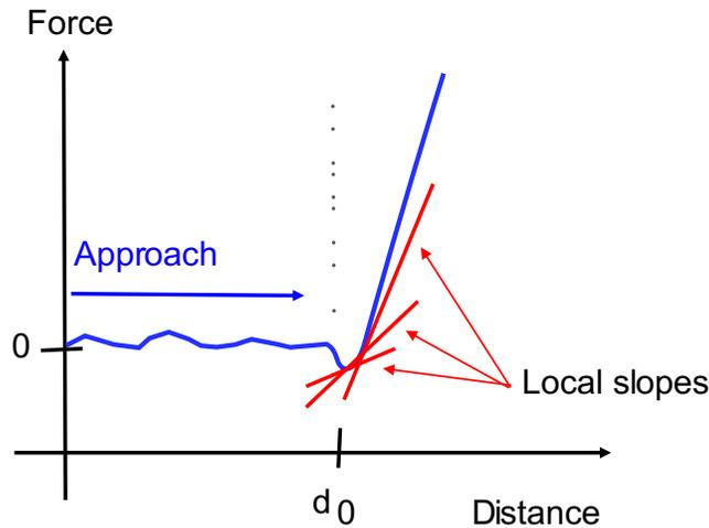
Figure 2: Schematic display of the stepwise analysis of a force-distance curve. Local slopes are marked in red. The indentation depth is calculated from the contact point  $d_0$ .
