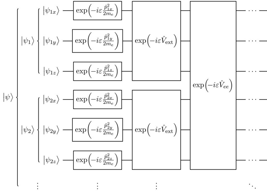
**Fig. 1** Overview of quantum circuit to implement unitary short time evolution,  $\hat{U}(\epsilon)|\psi\rangle$ , via Trotterization, on a quantum computer. This structure is used in both the canonical and CCS Trotter quantum circuitry.
