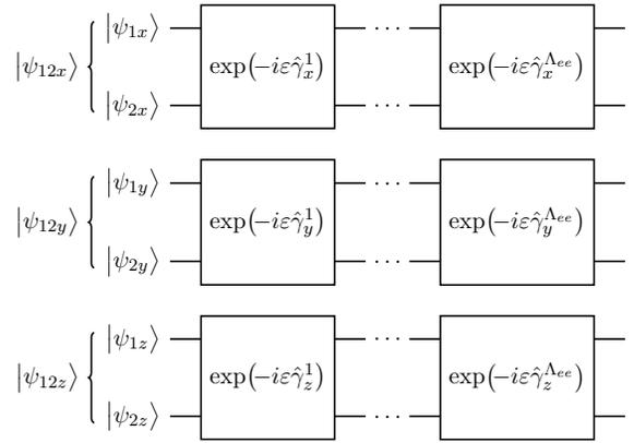
**Fig. 4** CCS quantum circuit to implement  $\exp(-i\varepsilon\hat{V}_{ee})|\psi_{12}\rangle$  on a quantum computer, based on Eq. (9). The six-dimensional  $V_{ee}$  function gate of Fig. 2 is now replaced with two-dimensional function gates, which separate by Cartesian component. The two-particle wavefunction contribution  $|\psi_{12}\rangle$  decomposes naturally into  $|\psi_{12x}\rangle$ ,  $|\psi_{12y}\rangle$ , and  $|\psi_{12z}\rangle$  components.
