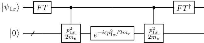
**Fig. 3** Quantum circuit to implement  $\exp\left[-i\varepsilon\frac{\hat{p}_{ix}^2}{2m_e}\right]|\psi_{1x}\rangle$  on a quantum computer. The function evaluation involves just a single coordinate (the momentum  $p_{1x}$ ), and hence just a single qubit set. This circuit is used in both the canonical and CCS Trotter quantum circuitry.
