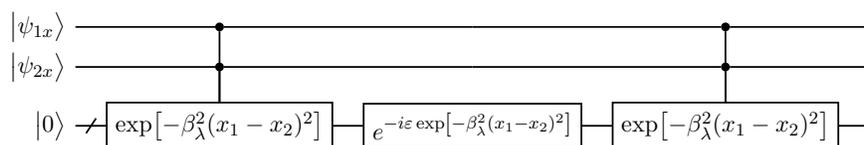
**Fig. 5** CCS quantum circuit to implement  $\exp(-i\varepsilon\hat{\gamma}_x^\lambda)|\psi_{12x}\rangle$  on a quantum computer, in the sinc DVR. The function evaluation,  $\gamma_x^\lambda = \exp[-\beta_\lambda^2(x_1 - x_2)^2]$ , involves two explicit coordinates and sets of qubits, and includes an exponential function evaluation.
