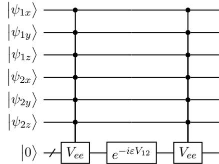
**Fig. 2** Canonical quantum circuit to implement  $\exp(-i\epsilon\hat{V}_{ee})|\psi_{12}\rangle$  on a quantum computer. The function evaluation,  $V_{12} = V_{ee}(x_1, y_1, z_1, x_2, y_2, z_2)$ , involves six explicit coordinates and sets of qubits, and includes an inverse square-root evaluation.
