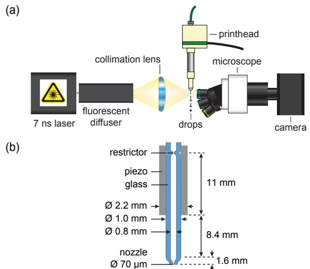
FIG. 3. (a) Experimental setup employed to image meniscus motion and bubble pinch-off in the drop-on-demand piezo-acoustic inkjet nozzle using illumination by laser-induced fluorescence (iLIF) [21]. (b) Schematic layout of the functional acoustic part of the inkjet printhead. It consists of a glass capillary tube (blue) that is tapered towards the  $70 \mu\text{m}$  nozzle exit. A cylindrical piezo (gray) can be actuated to drive the ink channel acoustics and the resulting droplet formation.
