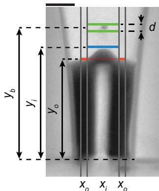
FIG. 4. Example of an image analysis result, showing the meniscus positions  $y_o$  of the outer region  $x_o$  and  $y_i$  of inner region  $x_i$ , the bubble position  $y_b$ , and the bubble diameter  $d$ . The scale bar represents 50  $\mu\text{m}$ .
