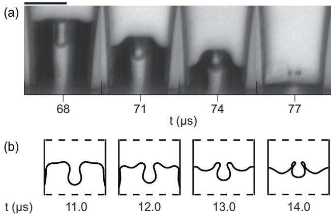
FIG. 9. (a) Toroidal bubble pinch-off as experimentally recorded for a rectangular pull-push pulse with an amplitude of 92 V and a width of 53  $\mu\text{s}$ . The scale bar represents 50  $\mu\text{m}$ . (b) Simulation using the BI method of the meniscus shape deformation process eventually leading to toroidal bubble pinch-off.
