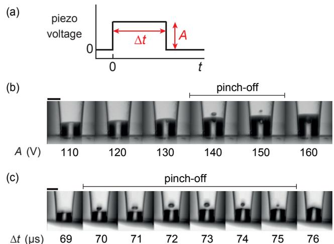
FIG. 2. (a) Rectangular piezo actuation pulse with its amplitude  $A$  and length  $\Delta t$  as the control parameters. Window of bubble pinch-off for (b) a pull-push pulse with a pulse width of 30  $\mu\text{s}$  and a varying amplitude, and (c) a pull-push pulse with an amplitude of 94 V and a varying pulse width. The scale bars represent 50  $\mu\text{m}$ .
