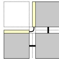
Fig. 2: The glue lengths used in our constructions: (1) length  $2\epsilon$  rigid bonds between cubic tiles, (2) length 0 rigid bonds between flat and cubic tiles, and (3) length  $3\sqrt{2}\epsilon/2$  flexible glues between flat tiles.
