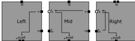
Fig. 29: Templates for the tile types which make up the first row of a **block** and allow the **block** to detach once the first row has completed. It is assumed that the first row of a **block** always grows from left to right. The “x” glues ensure that all tiles are bound with strength 2, and thus is it safe for the row to detach from the **genome** as soon as it completes. The rest of the **block** correctly grows from this row.
