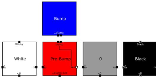
Fig. 26: Templates for tile types which make up a “bump” interface that extends in the same direction as the growth direction of the plane. These tile types are used for an interface that grows from left to right, so each “Pre-bump” tile stalls the growth of the interface until all of its associated “Bump” tiles have attached, ensuring that all “bumps” are in place before the Black tile is in place, since that allows the block to attach to a block with the complementary half of the interface.
