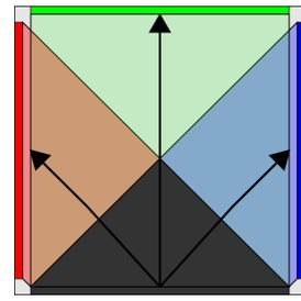
Fig. 23: Schematic of how information can be transmitted to three sides of one plane of a block, with rotations of alternating rows (as shown in Figure 22b) rotating information to the left and right sides.
