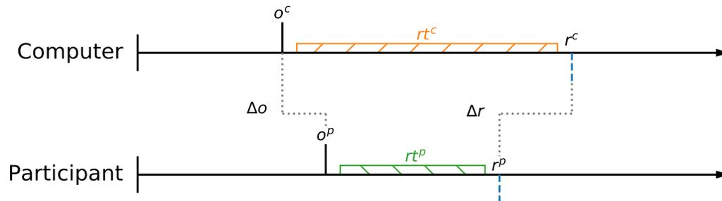
Note. In a common computer setup, response times are calculated from the onset and response times known to the computer ( $o^c$  and  $r^c$ , respectively). These times may differ from the actual onset and response times perceived and produced by the participant ( $o^p$  and  $r^p$ ). As a result, the obtained response time ( $rt^c$ ) is different from the one that is of interest ( $rt^p$ ).
