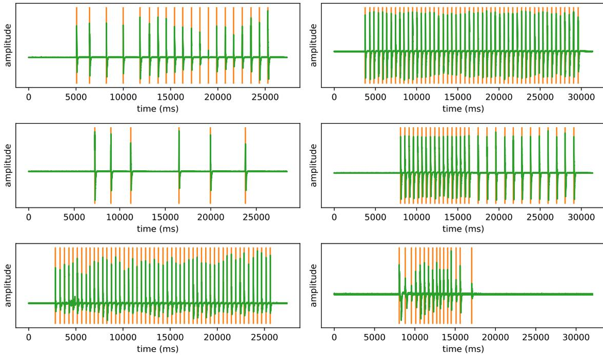
Note. Signal (green) is the activation of the input device (FSR) during one trial. Vertical lines (orange) are detected taps.
