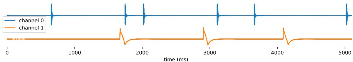
Note. The stimulus signal is an arbitrary stereo audio file (b). In this case, it is an audio signal constructed from designated onset times (a). The input recording (c) contains on one channel the looped-back signal from the stimulus (0) and on the other the electrical signal from the input device (1).
