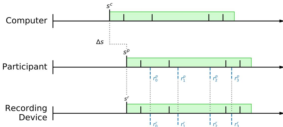
Note. This approach adds a new device that simultaneously records the stimuli and the responses with high accuracy. Stimuli are presented as one audio with multiple onsets (box containing lines). The stimulus presentation time may lag from the computer command but is recorded at the same time it is heard by the participant ( $s^c \geq s^p$  and  $s^p = s^r$ ). Response times ( $r_i$ ) are captured in synchrony with stimulus presentation.
