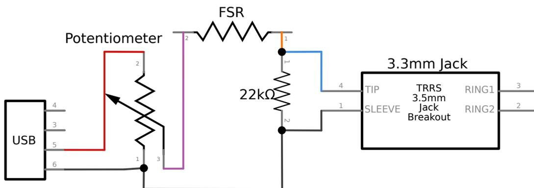
Note. The setup drives current with varying voltage from a VBUS pin of a USB (type-a) connector to the pin of a 3.5mm audio jack. Voltage is limited using a voltage divisor circuit (orange and purple). Final output voltage into the audio jack depends on the resistance provided by the FSR, that drops with pressure. The higher the pressure, the higher the voltage provided in the audio jack and recorded by the sound card. Schematic was drawn using Fritzing (Knörig, Wettach, & Cohen, 2009).
