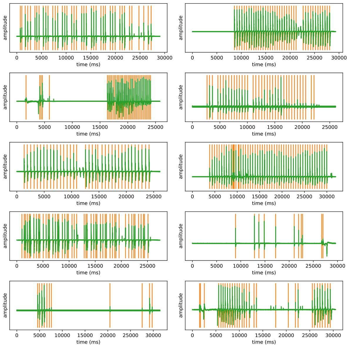
Note. Worst tap scenarios are considered as higher ratio of missing or spurious taps over detected taps. In most cases, missing taps are soft taps in comparison to the rest. Signal (green) is the activation of the input device (FSR) during one trial. Vertical lines (orange) are detected taps.
