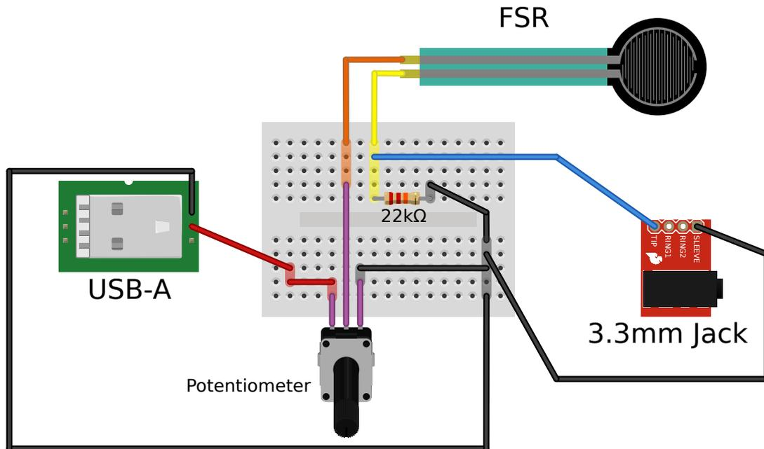
(b) Schematic of the electronic connections
