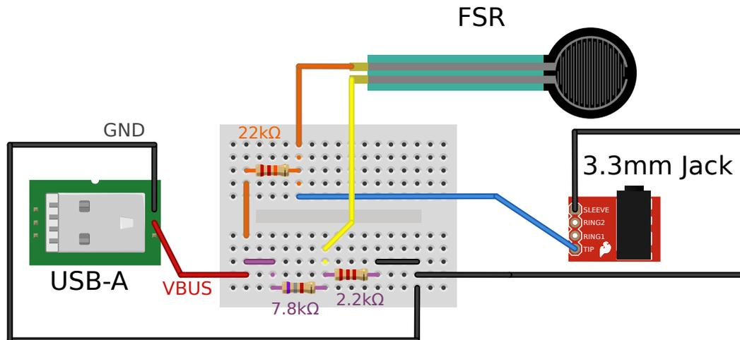
(b) Schematic of the electronic connections
