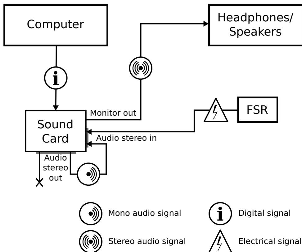
Note. Computer exchanges information with the recording device (sound card). One of the device's sound output is sent to the participant, the other has one channel looped-back to one of the recording device's input channels. The response device is connected to the other input channel.
