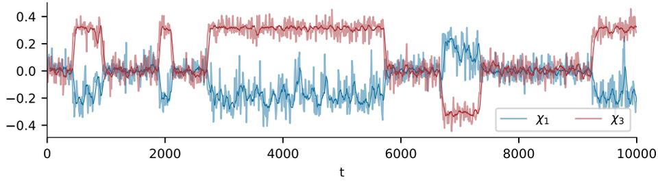
(a) Dynamics of first order cumulants  $\chi_i = \langle s_i \rangle$  (average over the population) in the intermittent regime QLE-NRC. Due to the  $g \rightarrow -g$  symmetry of the fitness function, two kind of trajectories are observed, mirrored with respect to zero - examples here are  $\chi_1, \chi_3$ . Solid blue/red lines represent the average over  $[t - \Delta t, t]$ , with  $\Delta t = 50$ . The NRC is characterized by  $|\chi_i| \sim \alpha$  for some  $0 < \alpha < 1$ .
