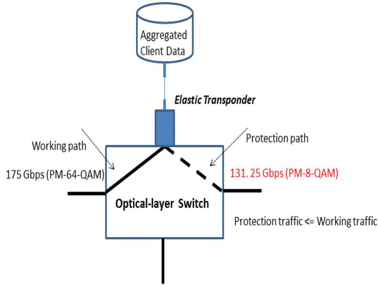
Figure 5: The optical node architecture supporting partial protection schemes
