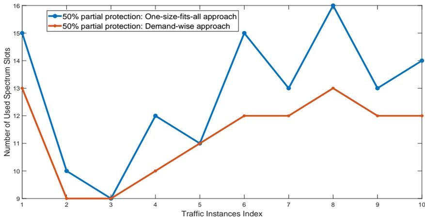
Figure 9: One-size-fits-all partial protection versus Demand-wise partial protection
