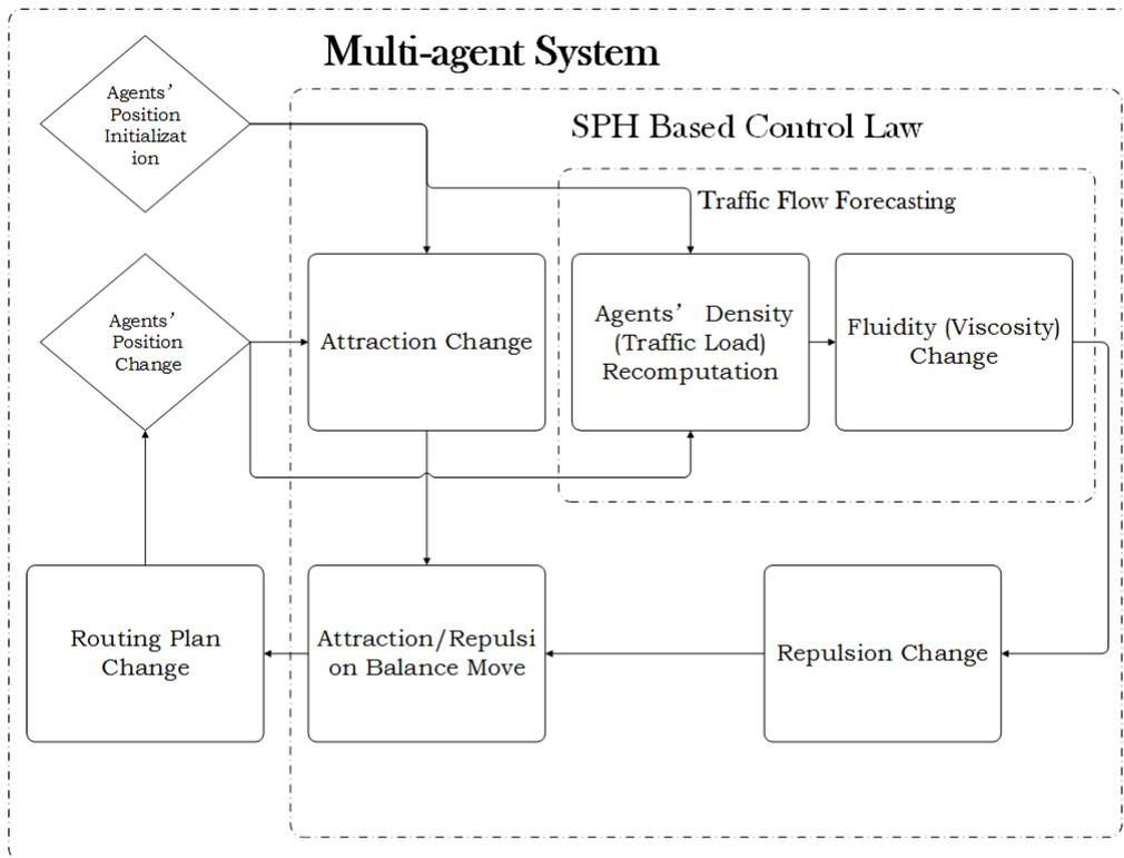
Fig. 1. Conceptual working diagram of our MAS based, SPH styled dynamic routing method
