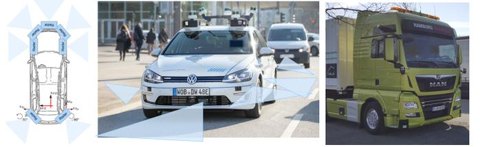
Fig. 3. Sensor setup of our vehicles. The cars use the 6 radars on the corners and on the sides, the trucks currently only 4: the two on the sides and on the front corners, respectively.
