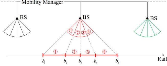
Fig. 3. Beam switching to get a LOS link.
