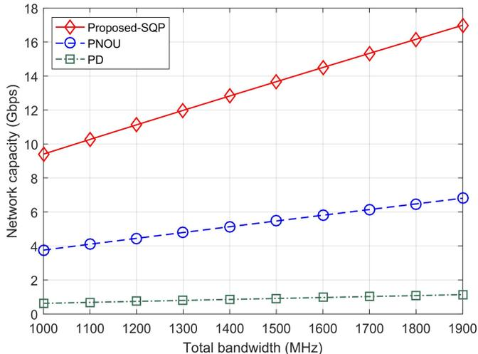
Fig. 5. Network capacity under different total bandwidth  $W$ .
