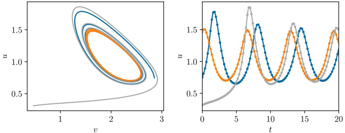
Figure 2: Dynamics of the Brusselator for  $a = 1$  and  $b = 2.1$ . As shown (through color) for three different initial conditions, the trajectories of the continuous-time dynamical system settle onto a limit cycle (left). Here, we sample the  $u(t)$  time series of such trajectories at discrete steps in time  $\delta t = 0.2$  apart, as illustrated on the right.
