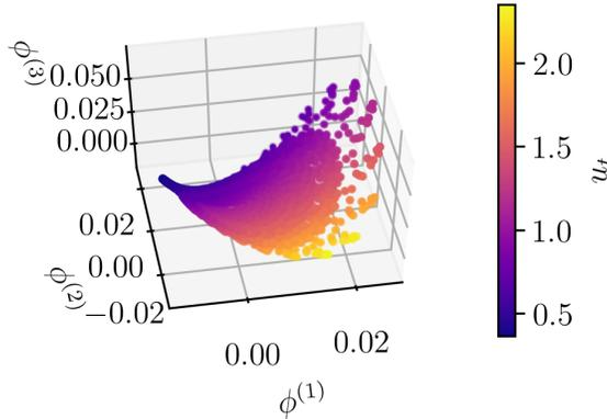
Figure 5: Data manifold obtained using diffusion maps on time series windows  $u_t$  of length  $l = 10$ , indicating that the data is in fact two-dimensional. The color encodes the initial value  $u_1$  corresponding to each window.
