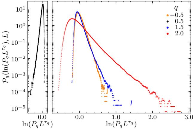
FIG. 19. Distribution  $\mathcal{P}_q(\ln[P_q(L)L^{\tau_q}]; L)$  at  $L = 1024$  for representative  $q$  values. The tail is seen to be approached from the peak value passing through an inflection point. Fig. 20 zooms into the tail.
