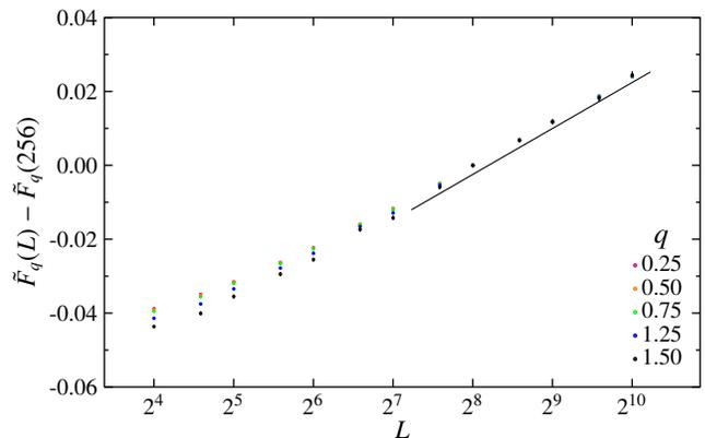
FIG. 17. The function  $\tilde{F}_q(L)$  displays a nearly perfect scaling collapse for all  $q$ -values listed (“hyper-collapse”). The finite slope of this trace is a manifestation of quartic terms in the multifractal spectra. The hyper-collapse indicates that corrections to quartic terms are very small in the regime of  $q$ -values here considered.
