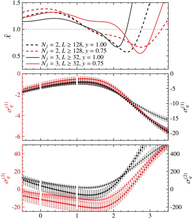
FIG. 28. Fit quality  $\tilde{\chi}$  as function of the moment  $q$  for a  $q$ -independent irrelevant exponent  $y$  for several fits with expansion order  $N_y$  and data ranges. Similar to the previous Fig. 27, the plot highlights that beyond a moment  $q_+$  finite-size corrections no longer follow the canonical expansion Eq. (12).
