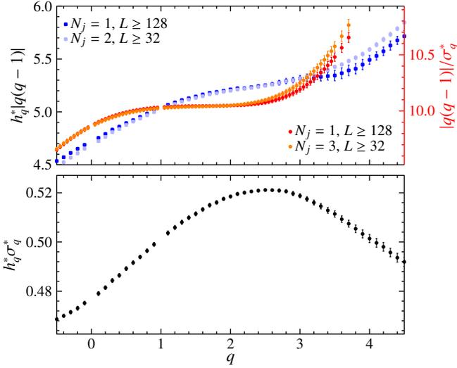
FIG. 18. Distribution height  $h_q^*$  and inverse width  $1/\sigma_q^*$  as function of  $q$ . The scaling by  $|q(q-1)|$  removes the trivial divergences and zeros at  $q = 0, 1$ . The two data sets are shown per observable in order to illustrate the goodness of the fitting, see Appendix VII B. The lower panel shows the effective area  $h_q^* \sigma_q^*$ .
