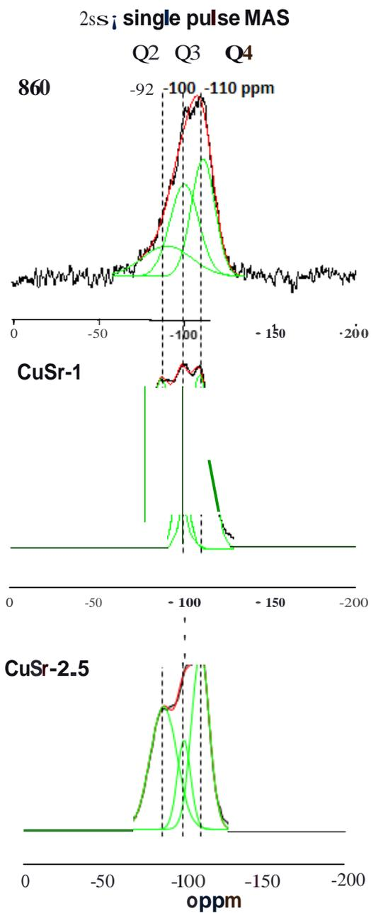
**Figure3.** Solid-state  $^{29}\text{Si}$  single-pulse MAS-NMR spectra of B60, CuSr-1 and CuSr-2.5 of B60, CuSr-1 and CuSr-2.5 samples. The areas for the Q<sup>n</sup> units were calculated by Gaussian line-shape deconvolution and are displayed in green.
