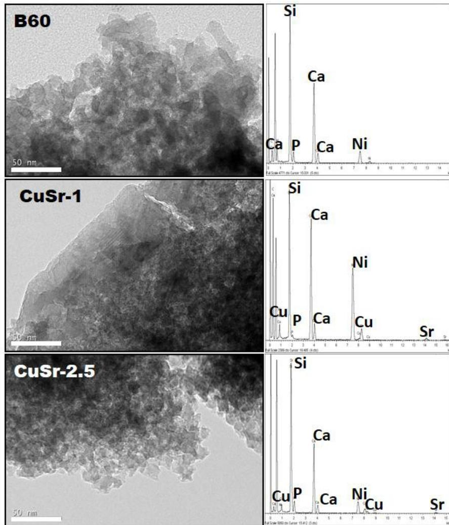
**Figure 1.** TEM micrographs (left) and EDX spectra (right) of B60, CuSr-1 and CuSr-2.5 bioactive glasses.
