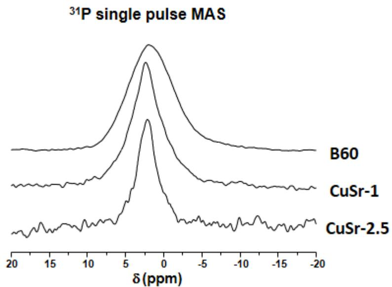
**Figure 4.** Solid-state  $^{31}\text{P}$  single-pulse MAS-NMR spectra of B60, CuSr-1 and CuSr-2.5 of B60, CuSr-1 and CuSr-2.5 samples.
