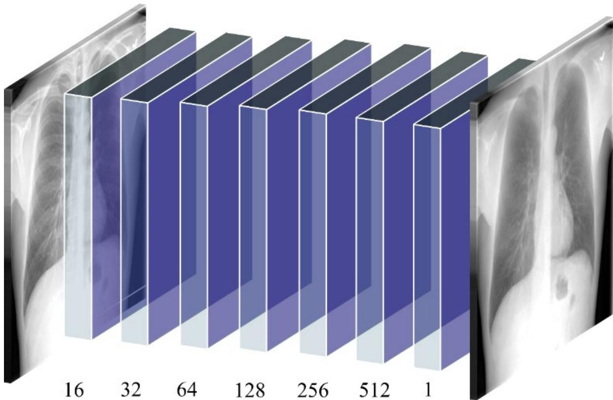
**Supplementary Figure 3.** The architecture of the proposed ConvNet-BS model. The ConvNet-BS model has seven convolutional layers (shown with blue-colored boxes) with zero paddings to preserve original input dimensions. The deepest convolutional layer with the sigmoidal activation produces bone-suppressed soft-tissue images.
