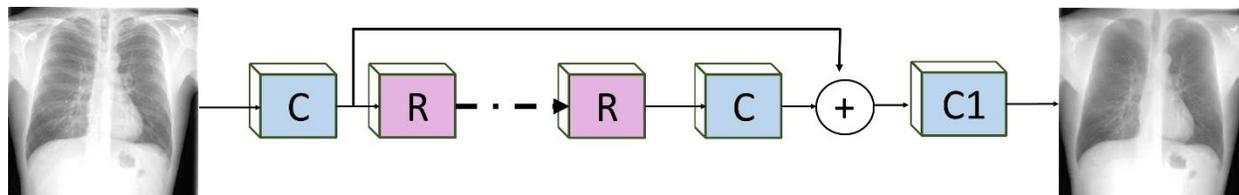
**Figure 1.** The architecture of the proposed ResNet-BS model. The convolutional block is denoted by C, having 64 filters of size  $3 \times 3$  and zero paddings to preserve input dimensions. R denotes the modified ResNet block where the final ReLU activation is removed together with the batch normalization layer. The proposed model has 16 ResNet blocks. The deepest convolutional layer C1 with a single filter, zero paddings, and sigmoidal activation, predicts the bone-suppressed image.
