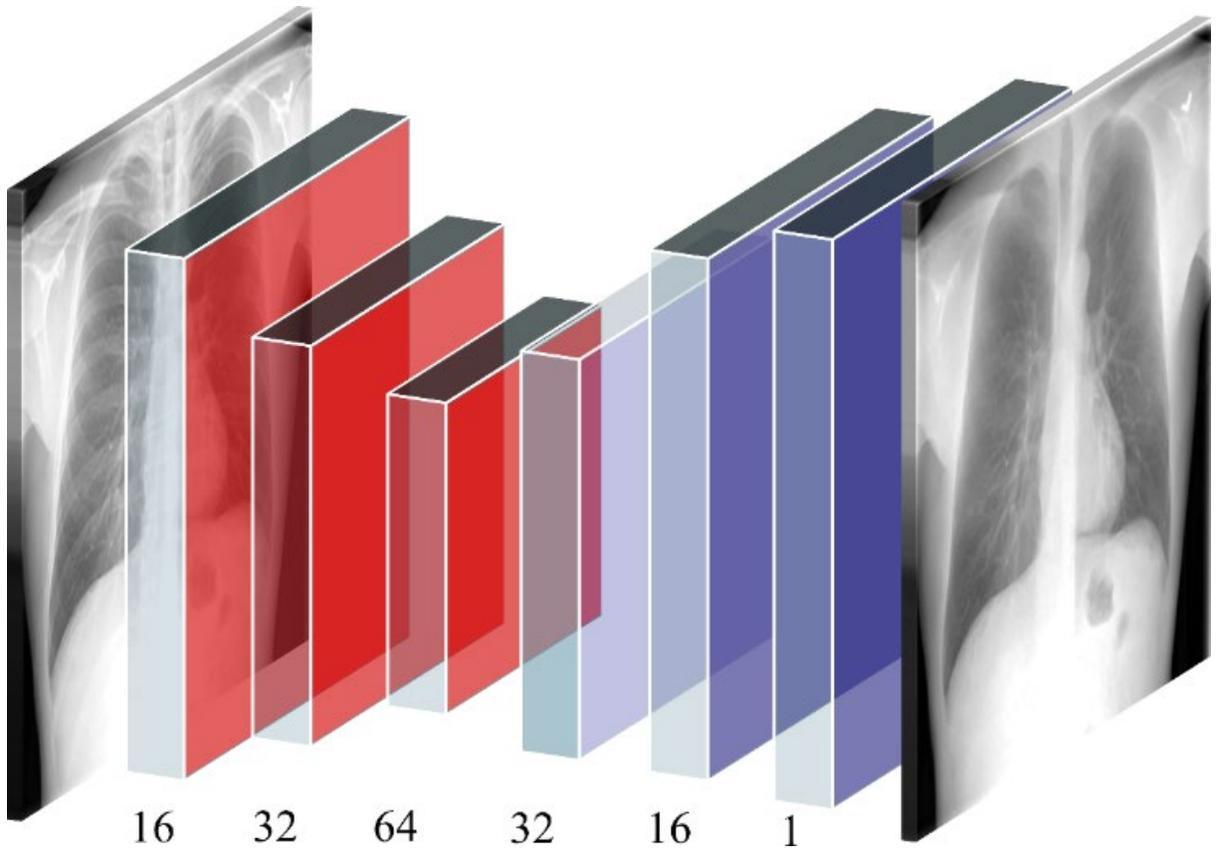
**Supplementary Figure 2.** The architecture of the proposed AE-BS model. The AE-BS model has a symmetrical convolutional encoder (shown with red-colored boxes) and decoder (shown with blue-colored boxes) architecture.
