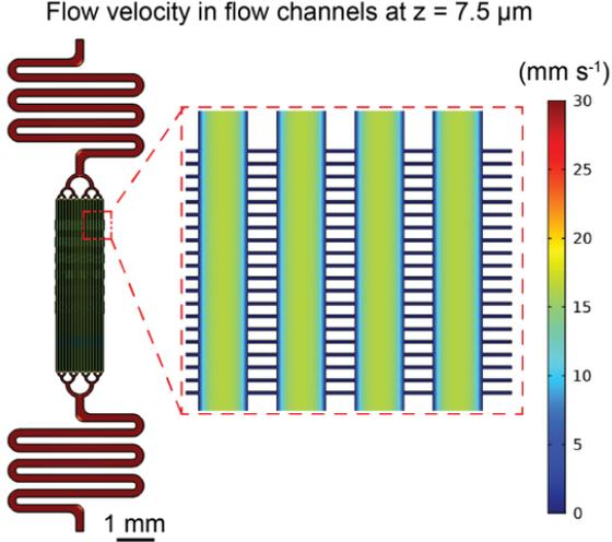
FIG. 12. Numerical simulation of the fluid flow in the PDMS microdevice. The dashed inset in red shows the magnified region in the chip where the flow channels have high flow velocity ( $16.2 \pm 0.3 \text{ mm s}^{-1}$ ).
