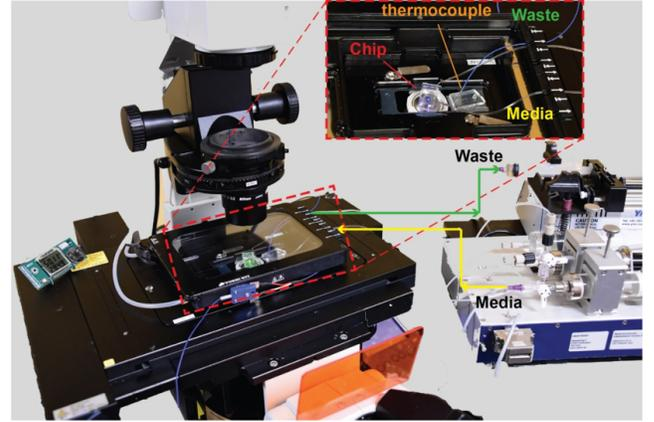
FIG. 14. The photo image of the microscopy setup. The inset shows the PDMS microdevice mounted in the on-stage temperature incubator. The M9 media was infused using a multichannel syringe pump and the waste was withdrawn using a syringe pump at early stage before the flow rate reached  $16 \mu\text{L min}^{-1}$  and then left open to atmosphere.
