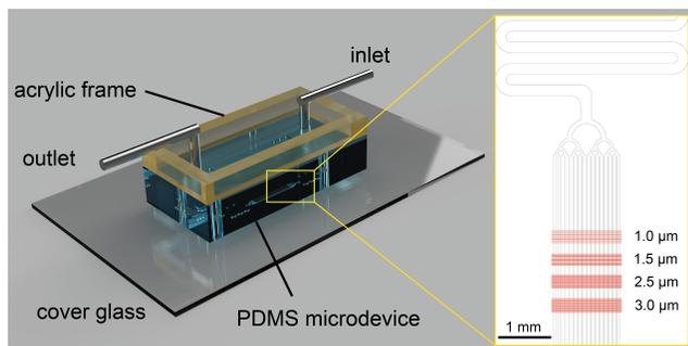
FIG. 8. Composition of the integrated microdevice used to track bacteria lineage in real time. The inset shows half of the symmetric design of microstructures in the PDMS device. The red pattern indicates the growth channels and the black pattern indicates the flow channels that are joined by a tree-like flow stabilizing structure and a flow resistor to an inlet or outlet.
