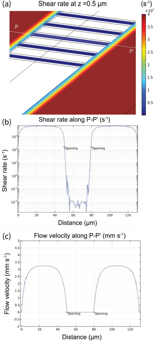
FIG. 13. The numerical simulation of fluid flow at the intersection of flow channels and growth channels. (a) The shear rate at the mid-plane ( $z = 0.5 \mu\text{m}$ ) of growth channel. (b,c) Data from the transverse line along P and P' on the side wall of the flow channels were extracted for quantification.
