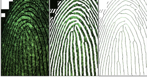
Figure 2. Fingerprint foreground, fingerprint ridge pixels, and the pixels used for generating the fingerprint ridge signal (left to right)
