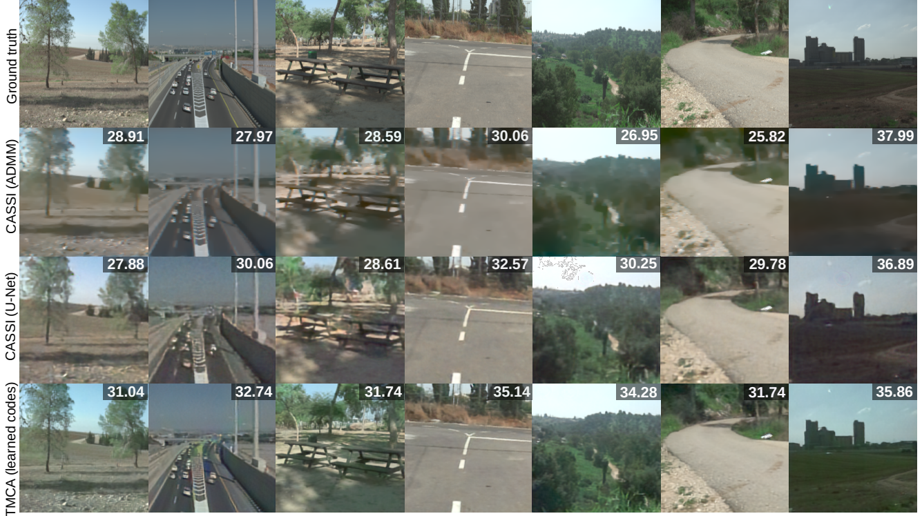
Figure S4. Additional results for compressive spectral imaging on the ICVL 1 test fold comparing our TMCA (fourth row) against the CASSI and using a conventional optimization technique (ADMM) as a decoder (second row) and a U-Net decoder (third row).
