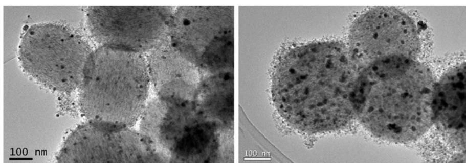
**Figure S2.** TEM micrographs of MSNs-AgBrNPs nanosystem.
