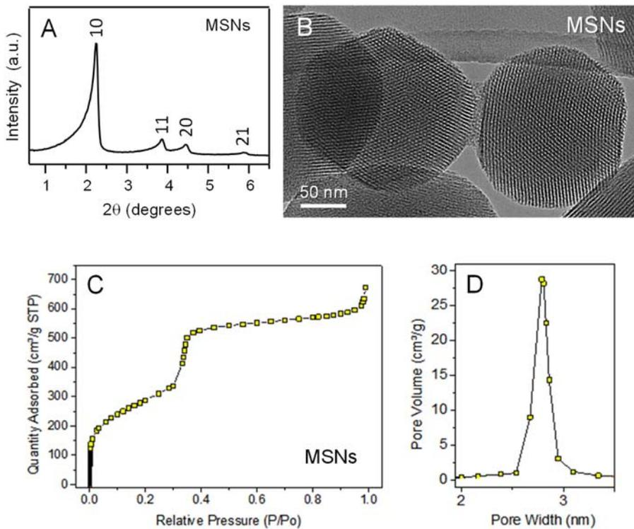
**Figure S3.** Characterization data of unmodified MSNs. A) Low angle powder X-ray diffraction pattern, B) TEM micrograph, C) N<sub>2</sub> adsorption-desorption isotherms and D) pore-size distribution. The textural parameters of the MSN materials obtained by N<sub>2</sub> sorption measurements are as follows:  $S_{BET} = 1054.9 \text{ m}^2/\text{g}$ ,  $D_p = 2.80 \text{ nm}$ ,  $V_T = 0.946 \text{ cm}^3/\text{g}$  and  $V_P = 0.854 \text{ cm}^3/\text{g}$ .
