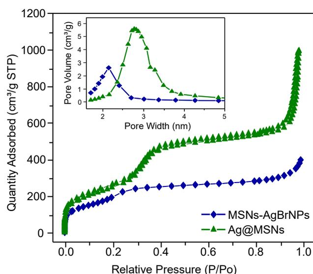
**Figure 4.**  $N_2$  sorption isotherms of MSNs-AgBrNPs and Ag@MSNs materials. The inset shows the corresponding pore size distributions for the mesoporous samples.
