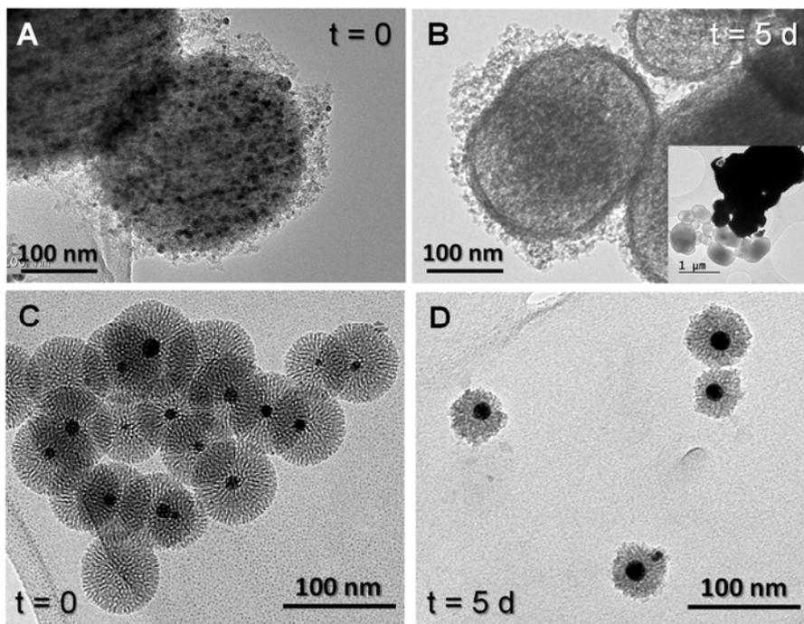
**Figure S6.** TEM images of MSNs-AgBrNPs (A, B) and Ag@MSNs (C, D) nanosystems before (A, C) and after 5 days of immersion in the *Mtb* culture medium (B, D).
