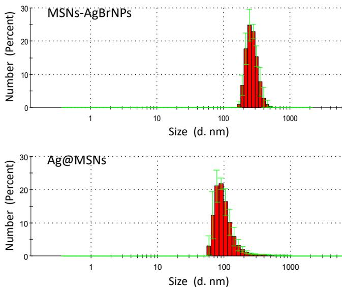
**Figure S4.** Hydrodynamic size distributions of materials measured by dynamic light scattering.
