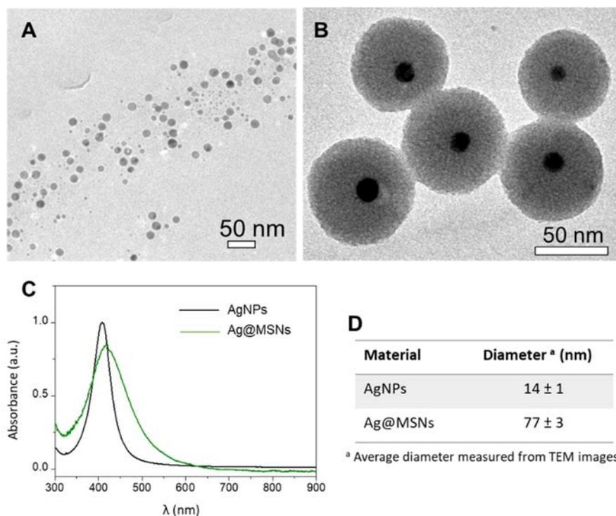
**Figure S1.** TEM micrographs of (A) silver nanoparticles and (B) surfactant containing Ag@MSNs. (C) UV-visible spectra of AgNPs in water and Ag@MSNs in ethanol. (D) Particle diameter obtained by measuring the nanoparticles in the TEM micrographs. Average diameters were calculated from 100 nanoparticles.
