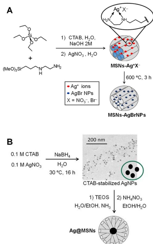
**Figure 1.** Scheme of synthesis of A) mesoporous silica nanoparticles containing silver bromide nanoparticles (MSNs-AgBrNPs) following a one-pot incorporation of silver ions and subsequent thermal treatment and B) core@shell type nanoparticles consisting of silver coated by mesoporous silica (Ag@MSNs).
