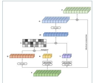
Figure 2 Illustration of the application of self-attention mechanism in speech enhancement GANs with  $L=9,\ C=6,\ p=3,$  and b=2.
