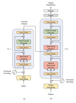
Figure 4 Model architecture of the Transformer. (a) Encoder (b) Decoder [36]
