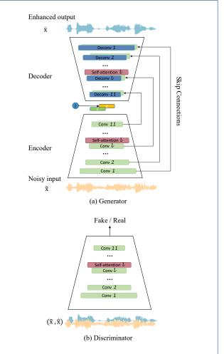
Figure 3 Illustration of the SA\_SEGAN architecture. (a) the generator component. (b) the discriminator component. [40]
