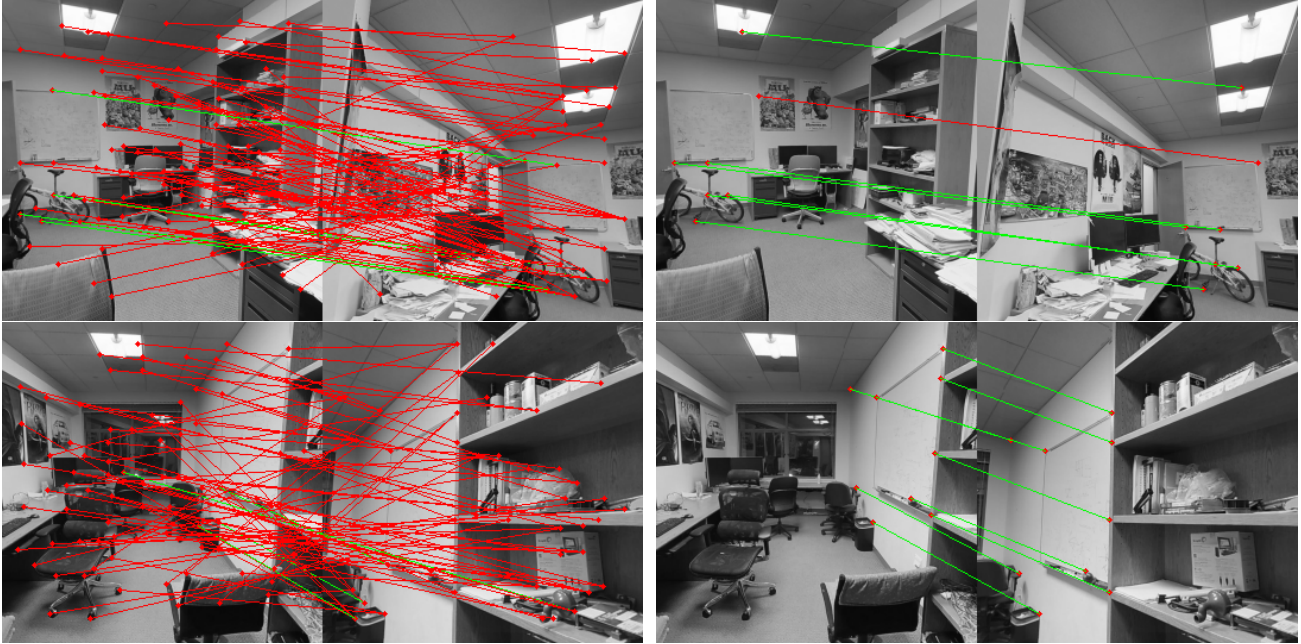
Figure 5. Examples of keypoint matching (Sec 4.1) with Superpoints (left) and our method (right). The inliers from the best pose estimated by RANSAC are in green and the outliers in red.
