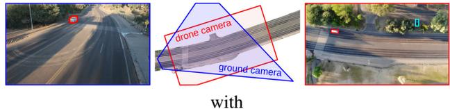
Fig. 7: Example images taken by the ground camera on the road infrastructure (left) and the drone at a height of 80 meters (right) at the second site. The coverage of both cameras are shown on the map (middle).
