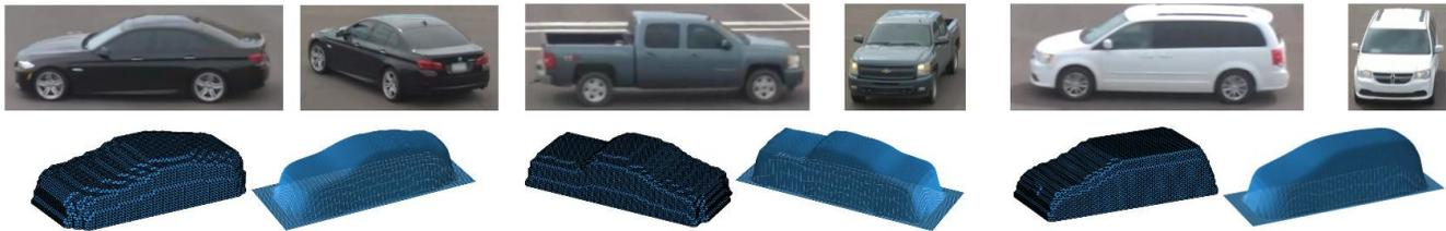
Fig. 9: Examples of reconstructed vehicles with voxel representations and histogram shapes.
