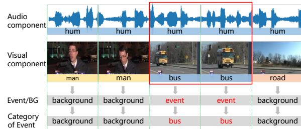
Figure 1. An illustration of the AVE localization task. Each video segment is composed of an audio and a visual component. In this example, the “hum” of the bus exists in all the segments (audio modality), but the visual images of the “bus” only appear in the third and fourth segments (visual modality). So only these two segments (red boxes) are localized as (bus) event, the remaining are recognized as background.
