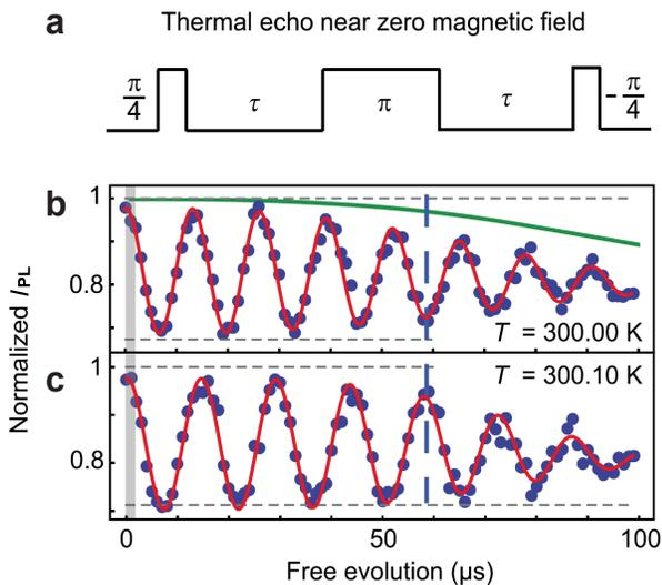
**Figure 4.** (a) Pulse sequence of thermal echo and (b) the resultant oscillations at two temperatures with NV centres in bulk diamonds (from [7]).
