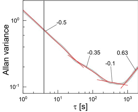
**Figure 6.** Allan variance profiles obtained from the steady temperature sensor signals as shown in the top panel in Fig. 3c. Slopes of the four distinct regions are indicated with values. The vertical line at 4 s indicates the tracking time used in this measurement (see Ref. [83] for details).
