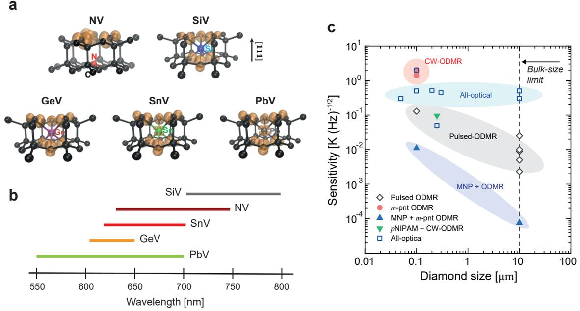
**Figure 1.** (a) Structures and spin polarization densities of spin defects in diamond for NV centres and group-IV colour centres (SiV, GeV, SnV, and PbV) (from [43]) and (b) their fluorescence spectral range. (c) Plots of temperature sensitivity vs. diamond size; data summarized in Table 1 with references. Notably, the sensitivity is dependent on the fluorescence photon count (or the optical excitation intensity). This brightness factor is not compensated in this figure.
