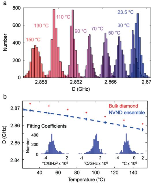
**Figure 8.** (a) Histograms of  $D$  as a function of temperature for NVND ensembles. (b) Mean value of  $D$  as a function of temperature for the NVND ensemble and bulk diamonds. (Inset) Histograms of the fitting coefficients (adapted from [103]).
