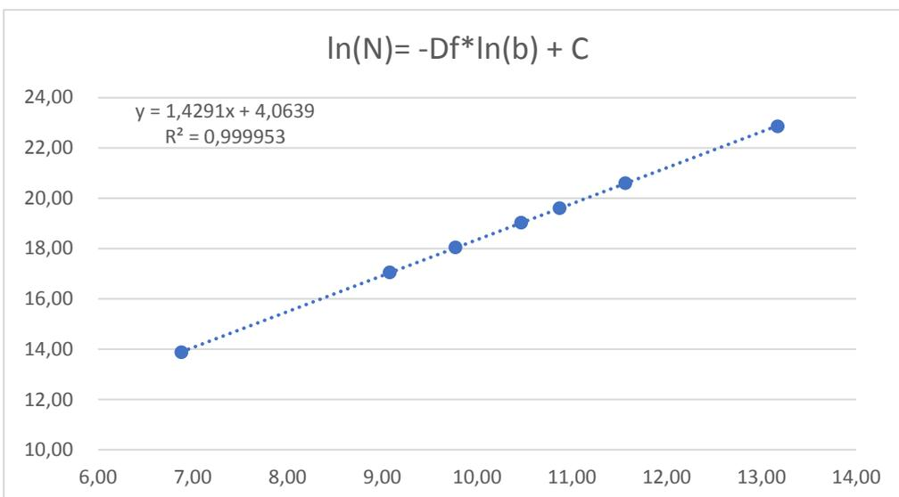
**Picture 3.** Linear regression applied for fractal dimension estimation.
