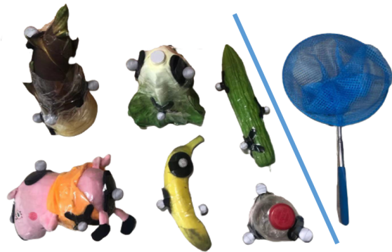
Fig. 6: The objects in the left are uneven objects we used for data collection. Infrared reflectors are fixed on objects for motion capture. Blue spoon net in the right is used as the basket. The Radius of spoon net is 10 cm.
