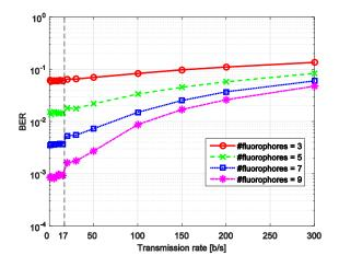
Fig. 2. Bit error rate as a function of transmission rate for communication between fluorophores and channelrhodopsins.
