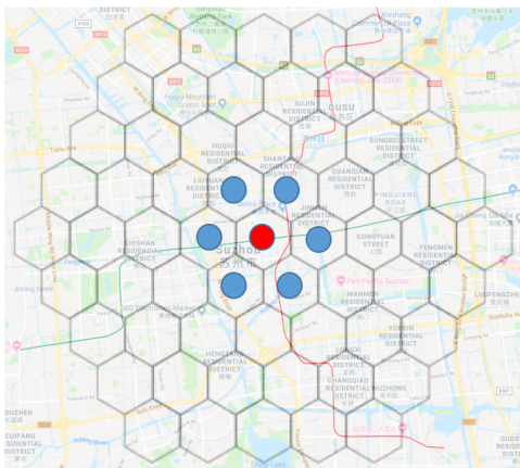
Figure 1: A sample map (obtained from Google Maps) overlaid with a hexagon grid system. The cell with a red circle represents the current cell of the vehicle, and those with blue circles are its neighboring cells.
