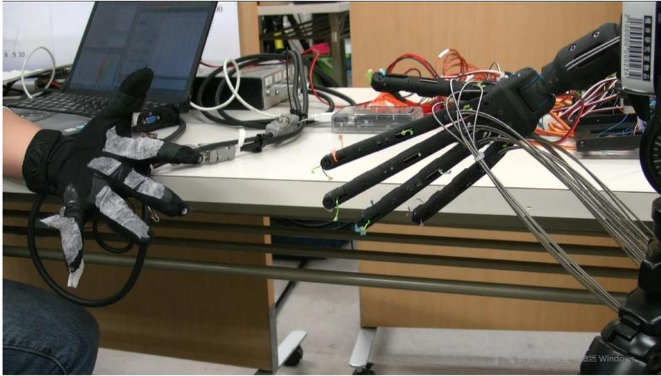
Fig.11 Test on the prosthetic hand arm robot system
