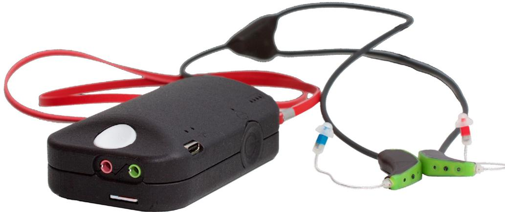
Fig. 3. The “Portable Hearing Laboratory” (PHL, [27]).
