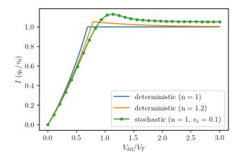
FIG. 4: Electrical current through each transistor in steady state conditions as a function of  $V_{\rm dd}$ .
